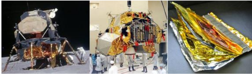
DuPont Kapton Polyimide (PI) Film External Insulated LEM (L); Internal LEM PI Insulation (C);PI Film Insulation Layering (R)
