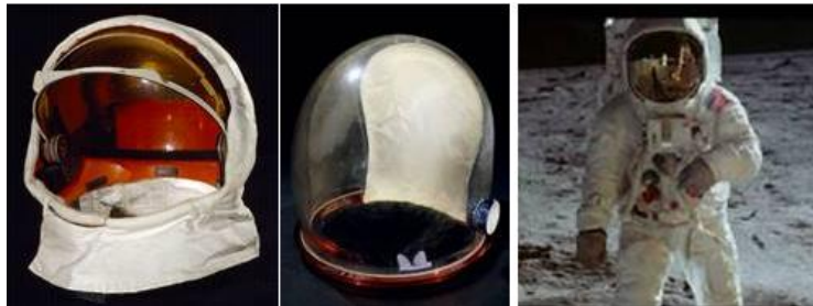
Extra-Vehicular Polysulfone Visor Assembly (L); Polycarbonate Pressure Helmet with White Temper Polyurethane Silicon Foam Cushioning (C); Neil Armstrong Moonwalking July 20, 1969 (R)
